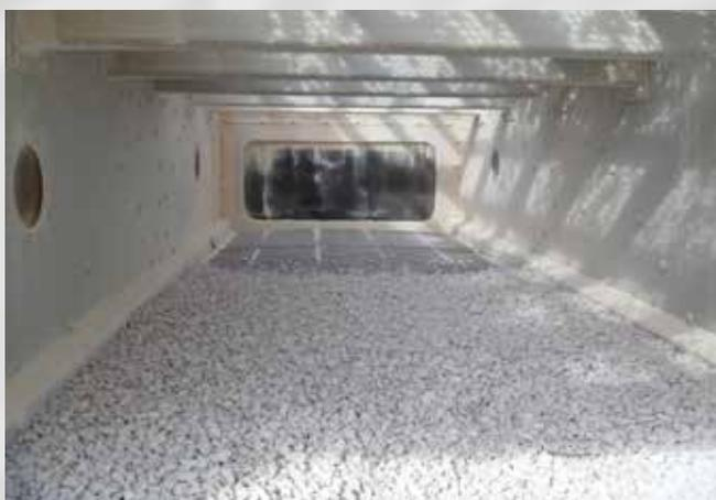
To always anticipate your requests, our aim was to create the horizontal Vibralto® screen, but also to innovate. Adding «Double Acceleration» made it possible for us to design a screen that can reach a record acceleration of 7.8g.
